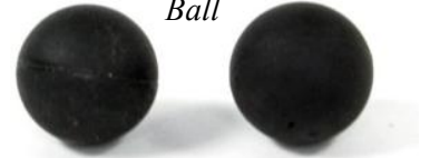
Crosslinked vs Not Crosslinked Rubber Ball
