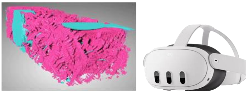
(left image) 3D distribution of Pb rich dendrites and voids in solders, captured by MA members using synchrotron measurements at the Advanced Photon Source at Argonne National Laboratory. (right image) Meta Quest 3 VR headset
