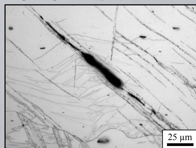
Fig. 6: Voiding in contraction twins (BF). \parallel ED. High \dot{\epsilon} .
