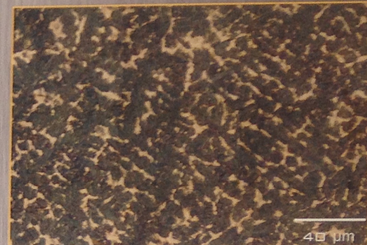
FIG. 4. Polarized LOM mosaic image of region A in Fig. 2, showing dendritic structures within the weld bead. Bainite has been formed within the dendrites, whereas the interdendritic regions are enriched in alloying elements and therefore remain austenitic.
