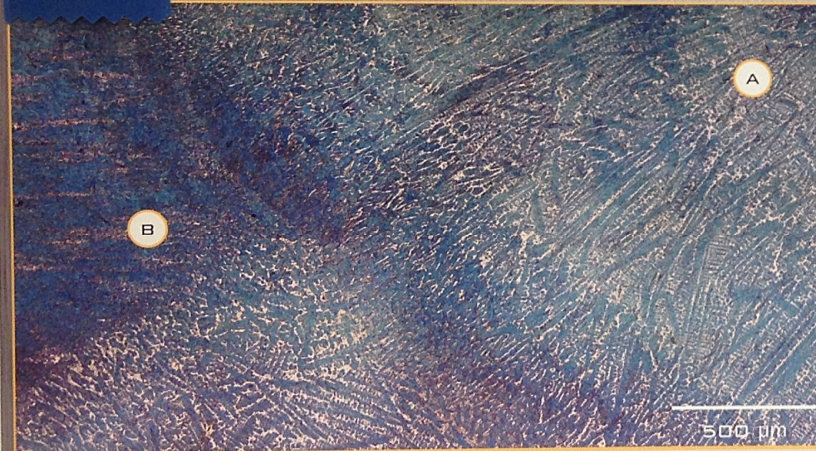
FIG. 2. Polarized LOM mosaic image of the junction point of the welds, marked as region 1 in Fig. 1. Visible are the dendritic structure of the weld (A), and the heat affected zone (B).
